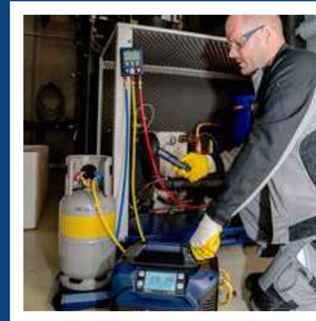
Connection hoses with ball valves for quick closing and opening of the refrigerant flow.
