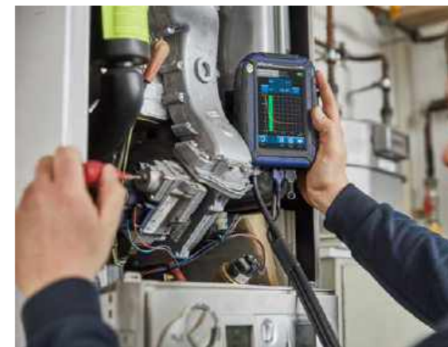
All values at a glance The tuning guide offers an advanced guidance to the technician to properly adjust the burner.
