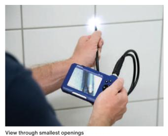
Just a Ø 6 mm opening in a tile cross is sufficient to view the installation behind the wall (in the picture Wöhler VE 320).
