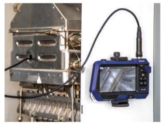
Hands free for working With the magnetic holder you can securely attach the Wöhler VE 400 to any magnetic surface. This leaves your hands free for working.
