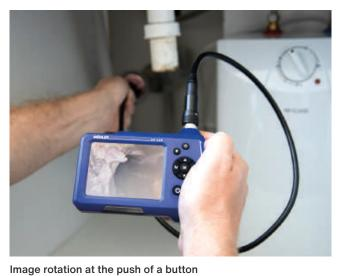
The display can be quickly rotated by 180° for easier navigation. The flexible probe easily passes bends.
